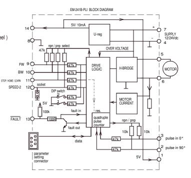
This is modified version from EM-241B or C Pulse counter block is added. This block can be used for end limit use.
