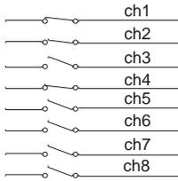
ALARM INPUTS 1 - 8 INPUT IMPEDANCE 10k. CAN BE CONTROLLED WITH CONTACT OR VOLTAGE SIGNAL
