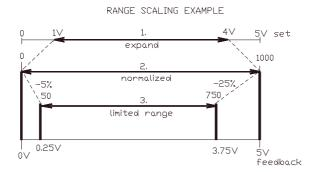
POSITION SET signal range is 1...4 $\vee$  Range is scaled with set parameters 21 = 100 and 22 = 400
