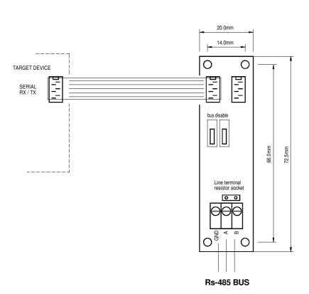
EM-P189 can be used to convert serial RX/TX to Rs-485 This card can be connected for EM- products which supports Modbus communication. Device includes the link cable compatible for EM- product.
