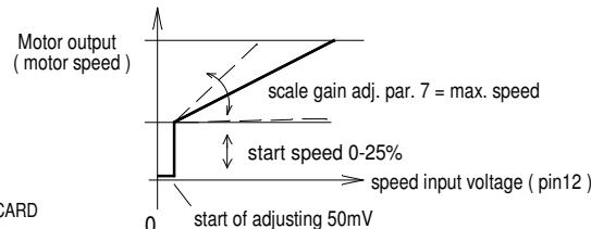
If symmetrical control is needed ( $\pm 5V$  or  $\pm 10V$ ), then an EM-A1 auxiliary card can be added into A1 slot. In symmetrical control the rotation direction determined by the polarity of the control signal and the middle point (0) is same as STOP. The installing of EM-A1 modified SPEED and DIR. inputs
