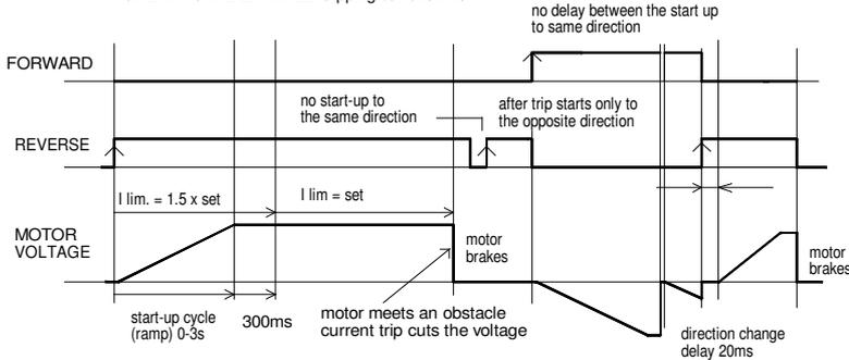
**OPERATION EXAMPLE: continuous current limit** (option start with impulse control - dashed line)
