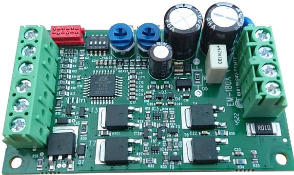
EM-180A is developed for controlled ON-OFF driving and direction change of a DC-motor with brushes. Driver has advanced current limit features. It limits the motor current in start-up and jam-situations and that way protects the motor and mechanics from over torque. Driver has also an error output to indicate error / over current situations.
