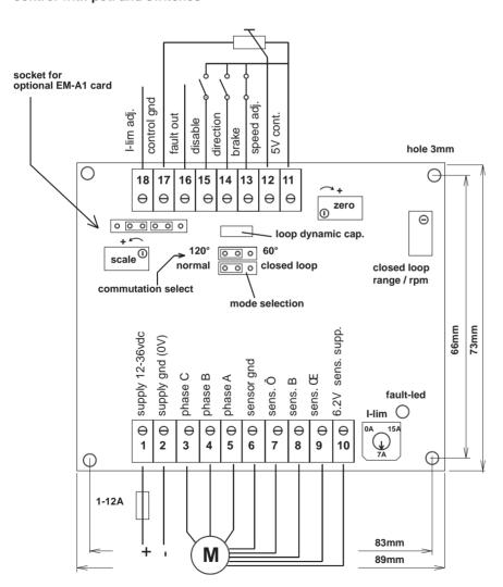
FAULT-output is pulled down and FAULT LED is lighted if at least one of the following conditions occurs:
