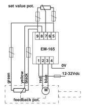
Spindle motor equipped with potentiometer, LINAK LA12
