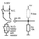
Examples for bias resistor switch res. 1k then R-bias 1k switch res. 2.2k then R-bias 1.8k switch res. 4.7k then R-bias 3.3k switch res. 10k then R-bias 4.7k
