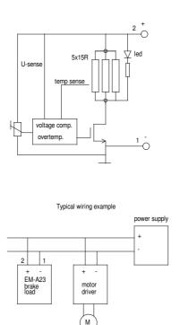
EM-A23 is a braking load for absorbing electric power. When motor slow down it degenerate energy, this energy will increase voltage level. This unit can be set to switch external resistor parallel to supply. Led on board will indicate that resistor is on. Unit has also over temperature protection.
