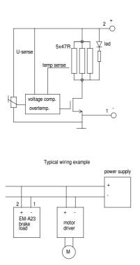
EM-A23-48V is a braking load for absorbing electric power. When motor slow down it degenerate energy, this energy will increase voltage level. This unit can be set to switch external resistor parallel to supply. Led on board will indicate that resistor is on. Unit has also over temperature protection.
